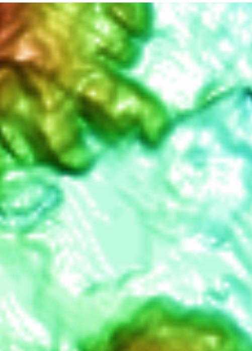
Space Imaging 2004 elevation image from a 20m topographic grid produced from stereo IKONOS satellite photos. The accuracy is between 5 and 10 meters of elevation.
