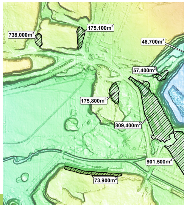
Penasquito mine site satellite elevation image February 27, 2010. The volumes of material removed from the pit and ore stockpiles between January 31 and February 27 are labeled. The accuracy of the measured elevation differences between the mapping dates is approximately 20cm.
