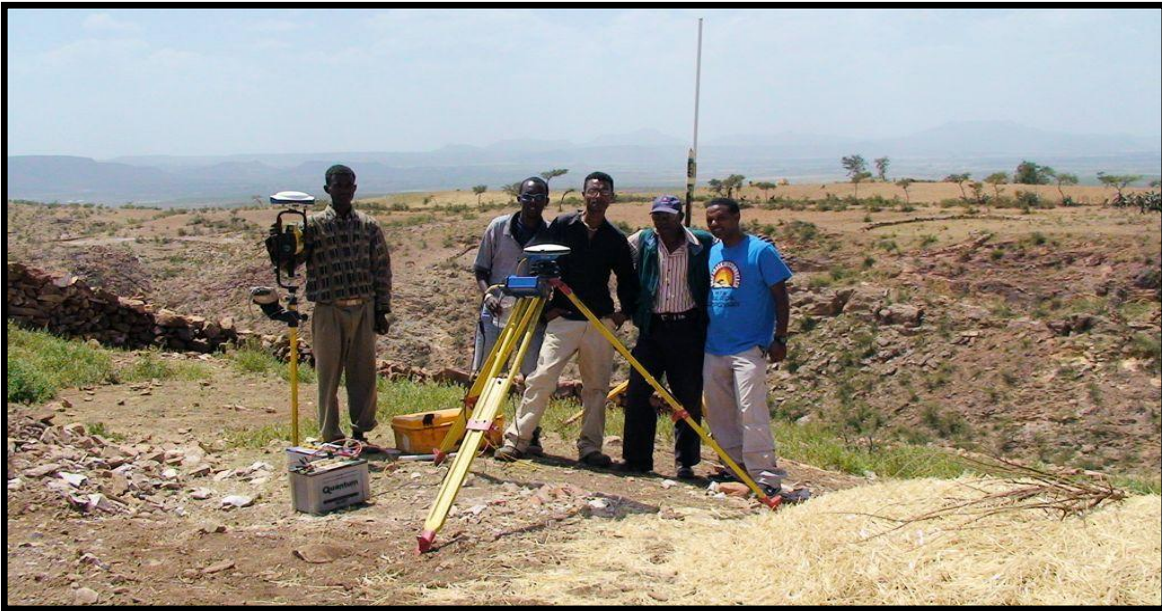
Figure 5. Asmara Eritrea. MWH Geo-Surveys differential GPS survey crew and equipment. Over 45,000 gravity stations were surveyed from 2004 through 2008 using differential GPS instruments from Magellan. All of the GPS positions were surveyed in Real Time Kinematic (RTK) mode with accuracies of 2 cm or better. 6,768 of these gravity survey stations were used as elevation checkpoints for the Cartosat-1 stereo satellite elevation mapping accuracy assessment. The Magellan RTK base with a ProMark™ 500 GPS rover are shown in this photo.
