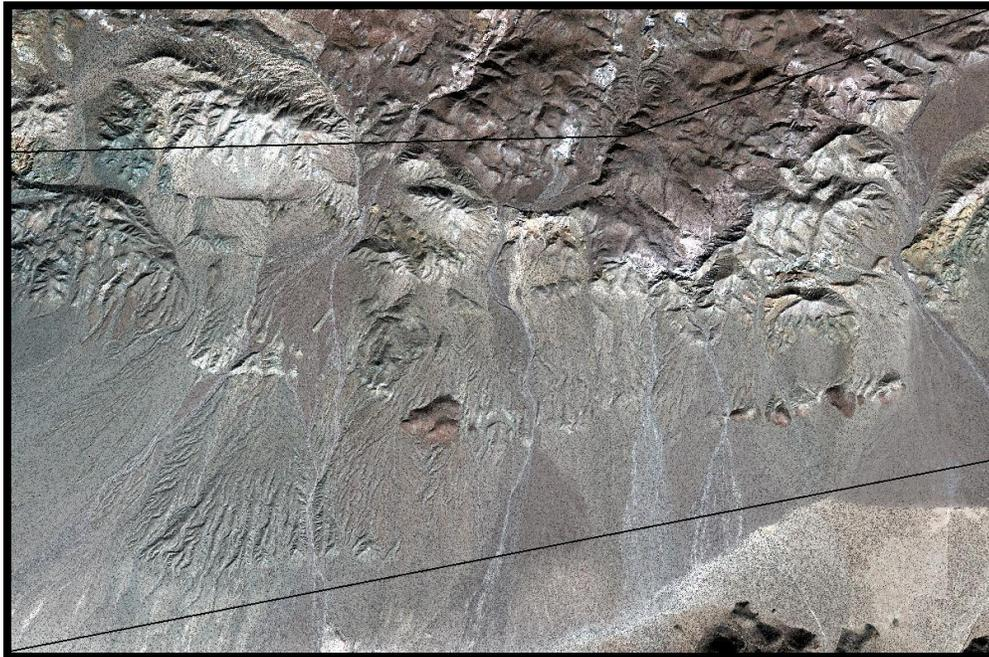
Figure 3. GeoEye-1 50cm resolution orthophoto, created from the GeoEye-1 stereo photos, for the area of the Garlock Fault LiDAR survey used in this study.
