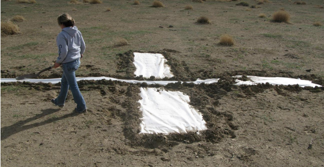
Figure 2a: This target is effective because it was created on even terrain, away from buildings and trees, and it contrasts the ground colour.
