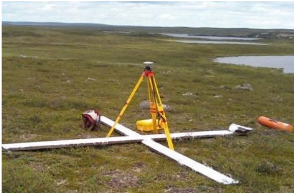
Figure 1a: This target is effective because it was created on even terrain, away from buildings and trees, it contrasts the ground colour, and the GPS unit is in the photo.
