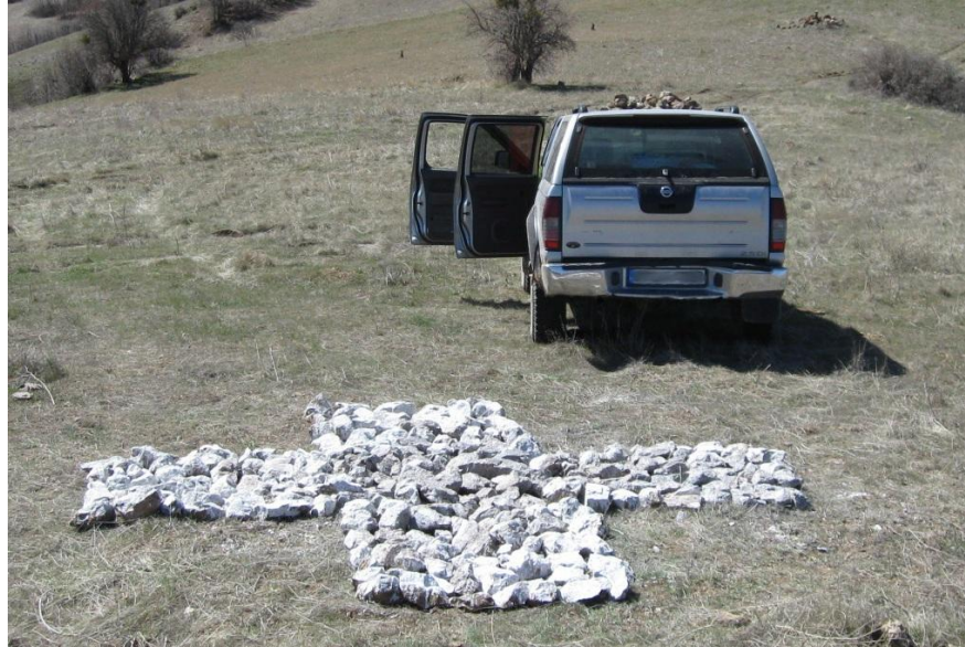
Figure 3a: This target is effective because it is away from buildings and trees, it contrasts the ground colour, and is made from solid, painted rocks that will not blow away or easily be destroyed.
