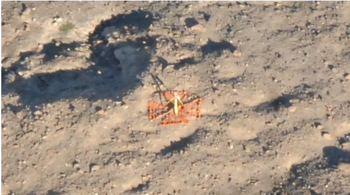
Figure 5a: This target appears clearly in the digital photo, but the contrast between the orange material and brown earth is not very strong.
