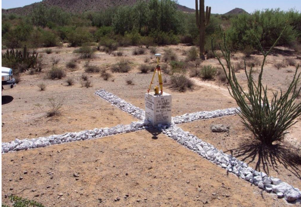
Figure 4a: This target is effective because it was created on even terrain, contrasts the ground colour, and is made from painted rocks that will not blow away or easily be destroyed. The target is clearly visible on the 50cm greyscale satellite image.
