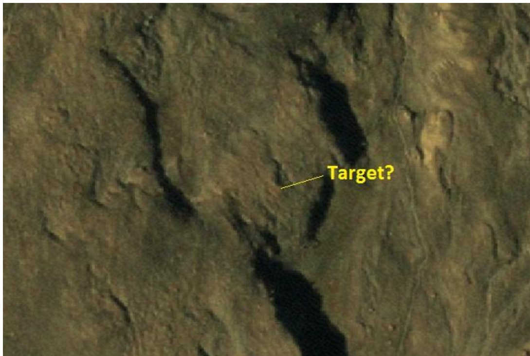
Figure 5b: The exact location of the target is not clear on the 50cm satellite photo because the orange colour blends into the brown background. A white target would have been more effective.
