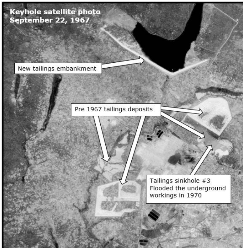
Figure 1. Declassified US Keyhole spy satellite photo of the Mfulira mine site and tailings dams taken on September 22, 1967.
