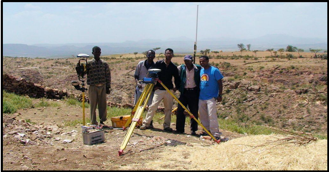
Figure 8. Asmara Project, Eritrea. MWH Geo-Maps differential GPS map crew and equipment. The Magellan RTK base with a ProMark™ 500 GPS rover are shown in this photo.
