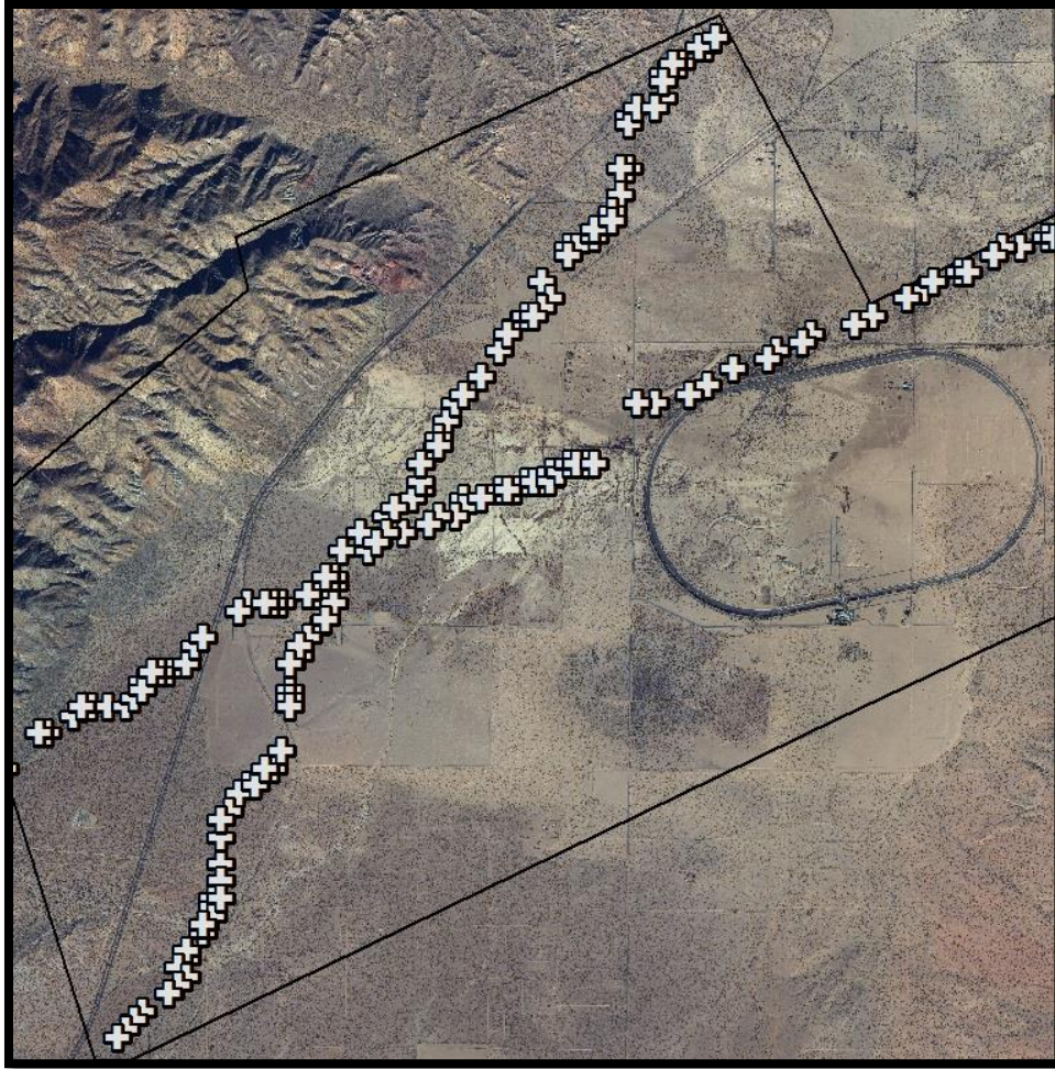
Figure 8. WorldView-3 50cm resolution orthophoto, created from the WorldView-3 stereo photos, for the area of the LiDAR survey used in this study. The 7.5 mile oval track is the Honda California Test Track.
