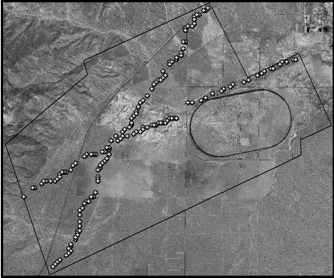
Figure 8. WorldView-1 50cm resolution orthophoto, created from the WorldView-1 stereo photos, for the area of the LiDAR survey used in this study. The 7.5 mile oval track is the Honda California Test Track. The 153 ground reference points are shown as a white crosses. The ground reference points were extracted from the LiDAR survey data. This distribution of survey points is typical of the survey points for source and receiver locations for 2D seismic surveys used in Oil and Gas exploration.
