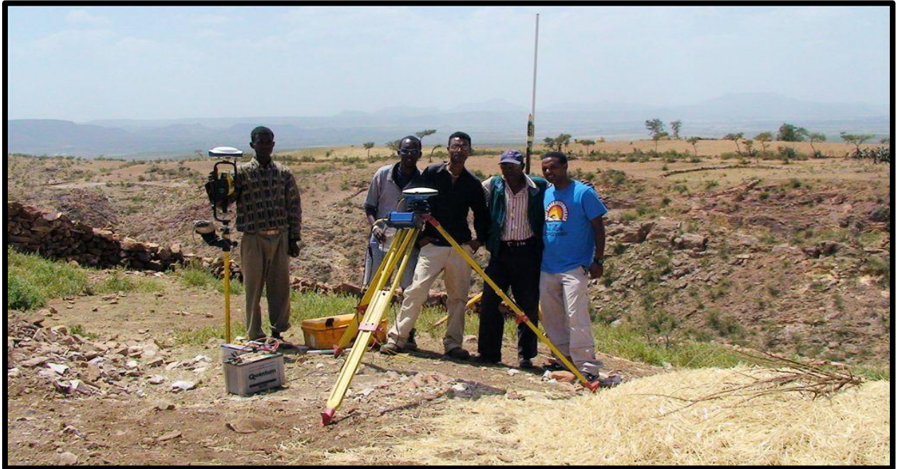
Figure 8. Asmara Project, Eritrea. MWH Geo-Surveys differential GPS survey crew and equipment. Over 45,000 points were surveyed from 2004 through 2008 using differential GPS instruments from Magellan. All of the GPS positions were surveyed in Real Time Kinematic (RTK) mode with accuracies of 2cm or better. 21 of these survey points were used as ground control points and 775 points were used as elevation checkpoints for this WorldView-2 stereo satellite elevation mapping accuracy assessment. The Magellan RTK base with a ProMark™ 500 GPS rover are shown in this photo.
