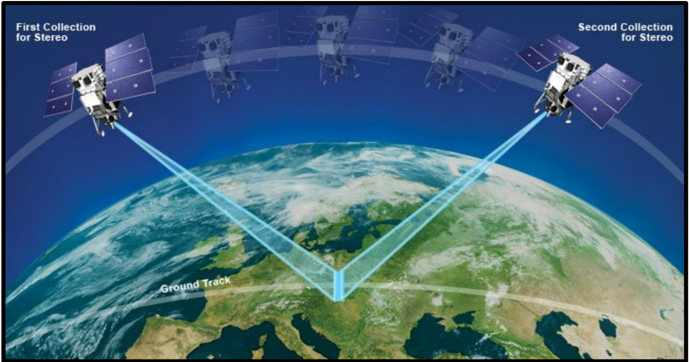
Figure 4. Illustration showing the process of taking satellite stereo photos. The satellite points forward to take the first photo. About one minute later, and 300 km further along its orbital track, the satellite rotates to take the second photo looking backwards along the track. Hundreds of km 2 can be accurately surveyed with a single pair of stereo satellite photos.
