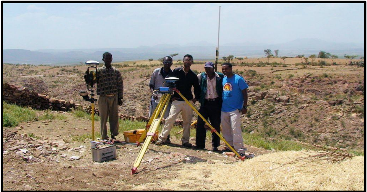
Figure 8. Asmara Project, Eritrea. MWH Geo-Surveys differential GPS survey crew and equipment. Over 45,000 points were surveyed from 2004 through 2008 using differential GPS instruments from Magellan. All of the GPS positions were surveyed in Real Time Kinematic (RTK) mode with accuracies of 2cm or better. 21 of these survey points were used as ground control point and 881 points were used as elevation checkpoints for the WorldView-3 stereo satellite elevation mapping accuracy assessment. The Magellan RTK base with a ProMark™ 500 GPS rover are shown in this photo.
