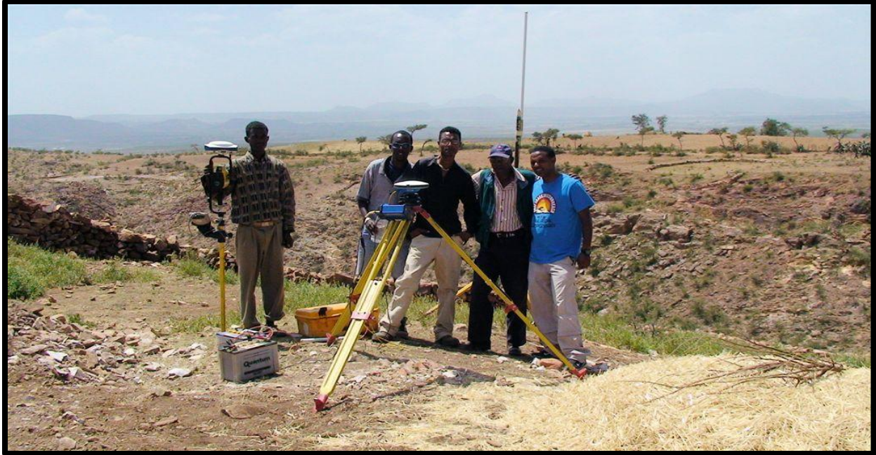
Figure 10. Asmara Project, Eritrea. MWH Geo-Surveys differential GPS survey crew and equipment. The Magellan RTK base with a ProMark™ 500 GPS rover are shown in this photo.
