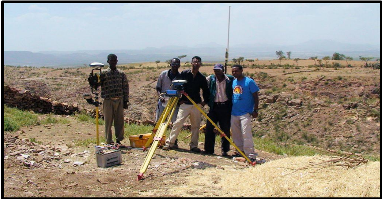
Figure 9. Asmara Project, Eritrea. MWH Geo-Maps differential GPS map crew and equipment. The Magellan RTK base with a ProMark™ 500 GPS rover are shown in this photo.
