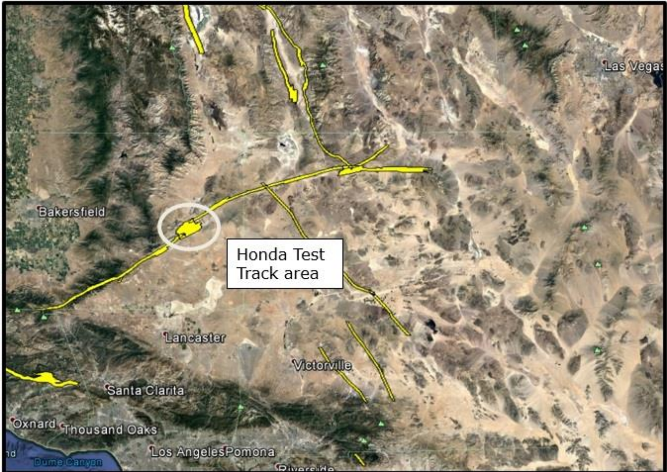
Figure 2. The Garlock Fault OpenTopography LiDAR survey shown on Google Earth. The Garlock Fault LiDAR survey was flown in April, 2008. The location of the WorldView-1 stereo satellite photos, acquired June 20, 2010, is shown by the circle.
