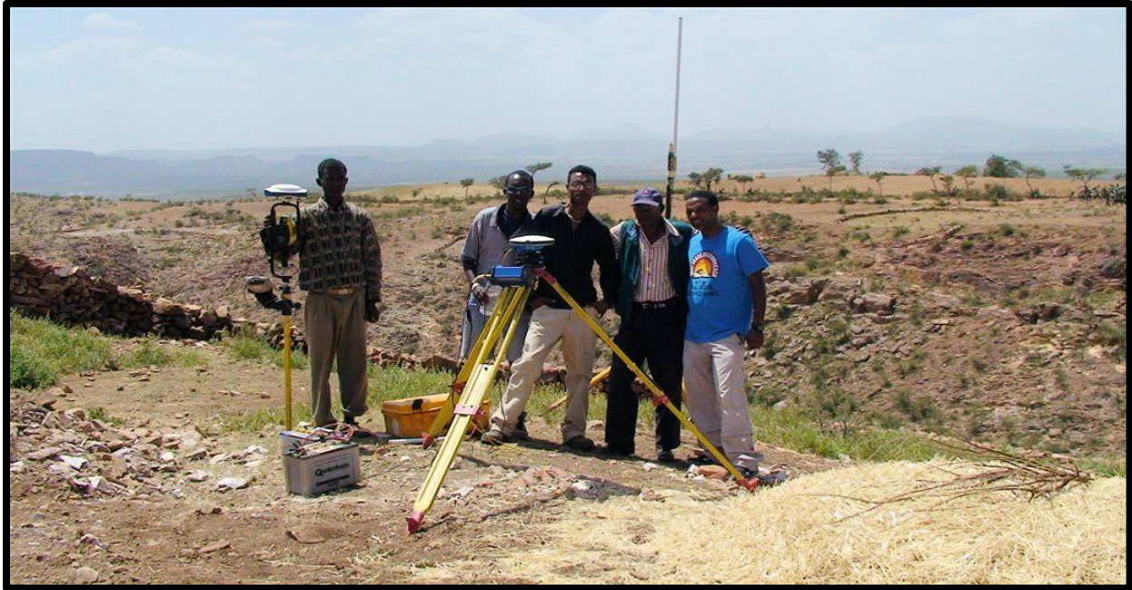
Figure 9. Asmara Project, Eritrea. MWH Geo-Survey differential GPS survey crew and equipment. The Magellan RTK base with a ProMark™ 500 GPS rover are shown in this photo.
