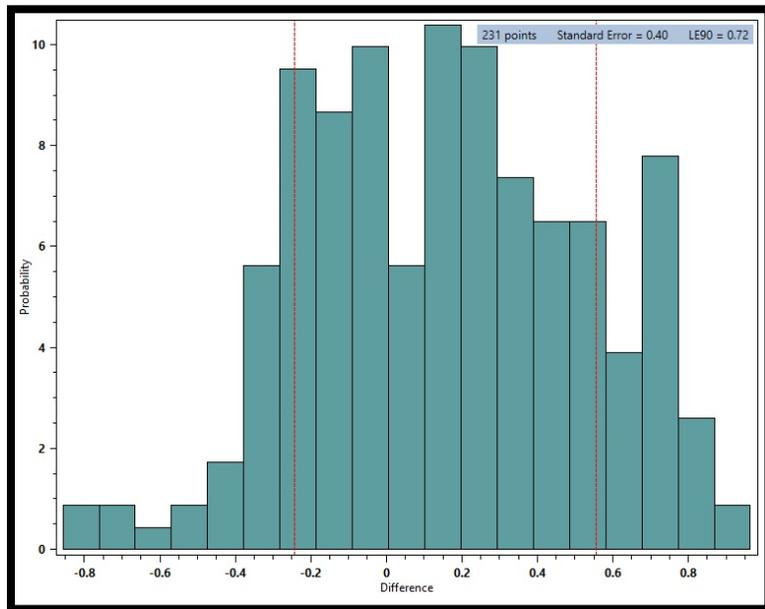
**Figure 12.** Histogram of the elevation differences between the Pleiades-1B stereo satellite elevations for the 14.4km by 13km area and the 231 elevation checkpoints with slopes between 20% and 100% grade. RMSE 40cm, LE90 72cm.
