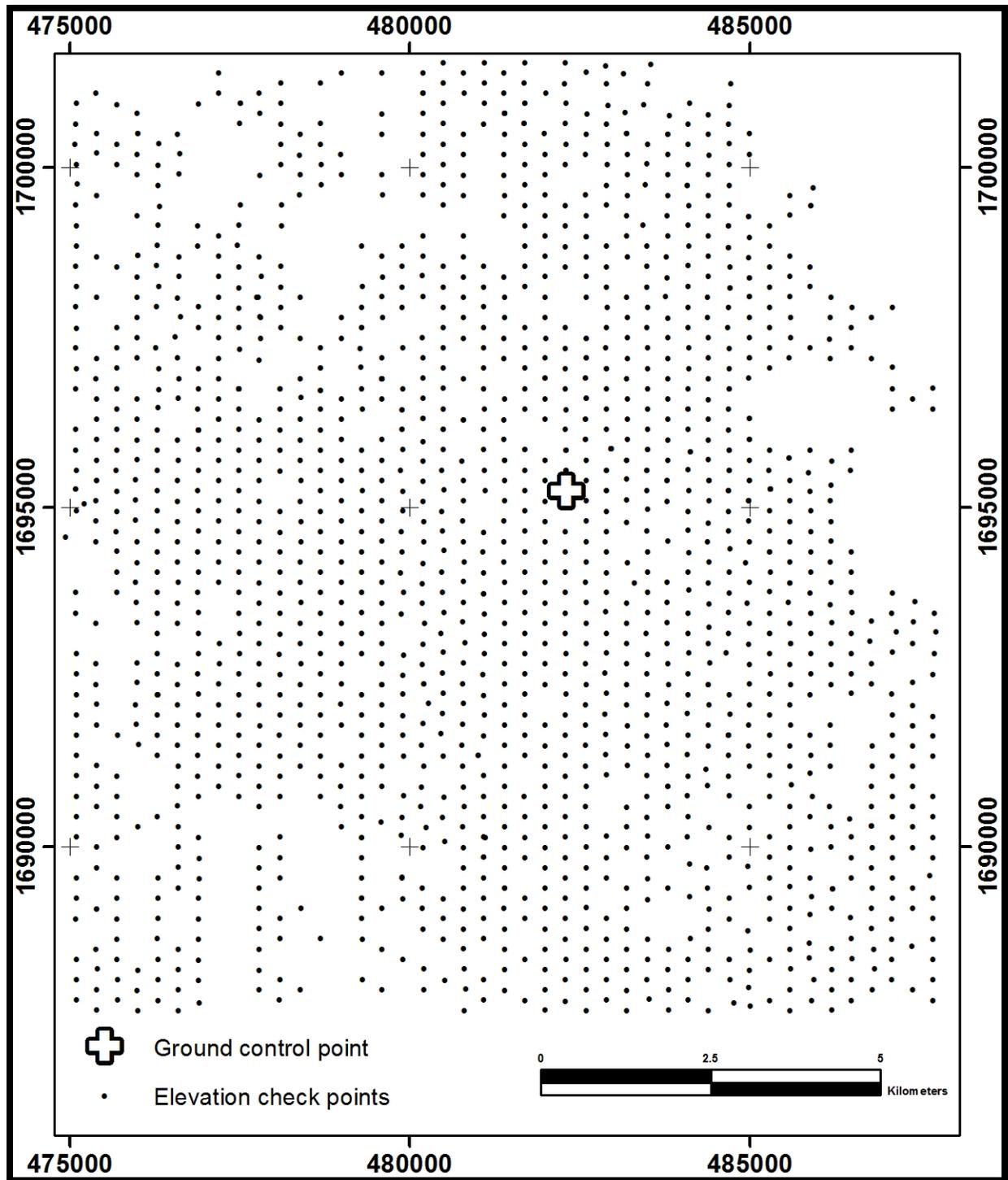
**Figure 8.** Area of the 14.4km by 13km Eritrea Stereo Pleiades-1b 1m elevation grid showing the ground control point and the 1,677 gravity survey stations used as elevation checkpoints to determine the accuracy of the stereo satellite survey.
