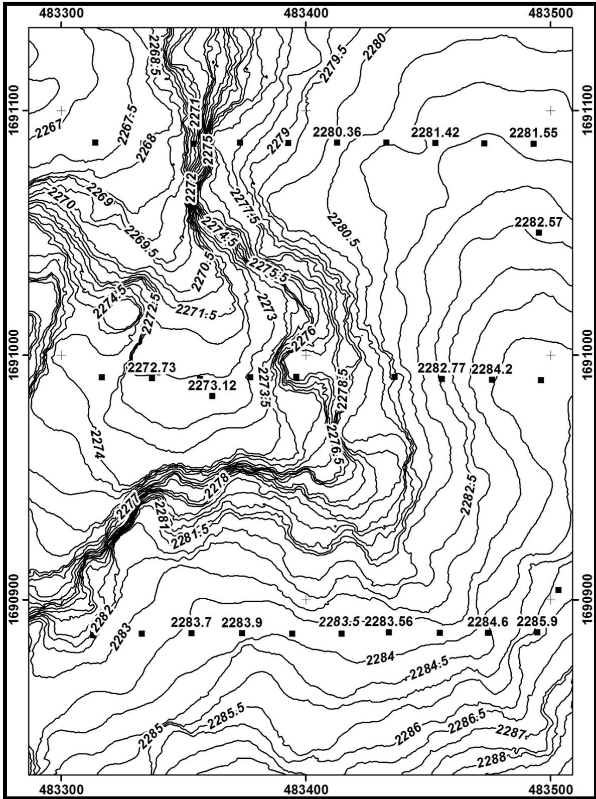
**Figure 13.** 50cm contours from the stereo Pleiades-1B elevation survey showing the elevations of some of the elevation checkpoints used to determine the stereo satellite elevation surveying accuracy of 28cm RMSE.
