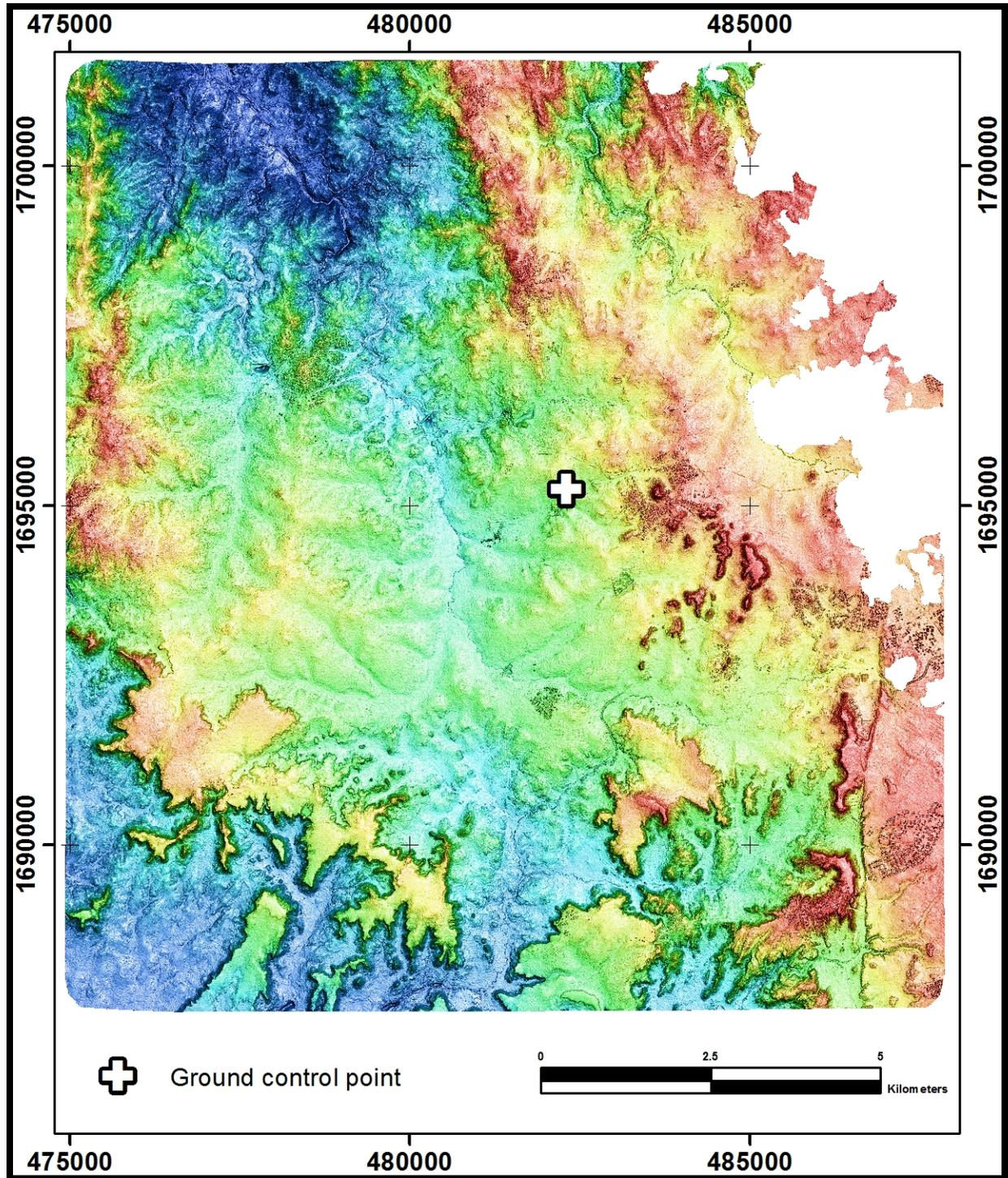
**Figure 7.** Stereo Pleiades-1B elevation image created from the 1m PhotoSat Asmara, Eritrea satellite survey grid. The figure shows the location of the ground control point.
