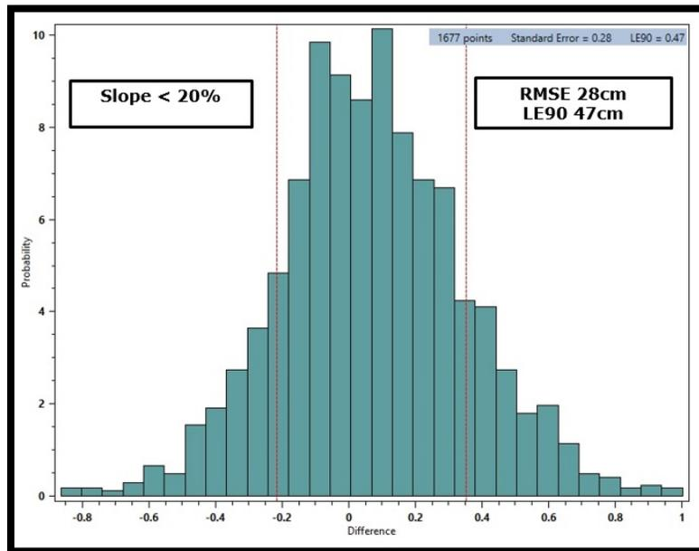
**Figure 10.** Histogram of the elevation differences between the Pleiades-1B stereo satellite elevations for the 14.4km by 13km area and the 1,677 elevation checkpoints with slopes less than 20% grade. The *Guidelines for Digital Elevation Data* of the US National Digital Elevation Program (NDEP) recommends that elevation checkpoints should be chosen in areas with slopes less than 20% grade. RMSE 28cm, LE90 47cm.
