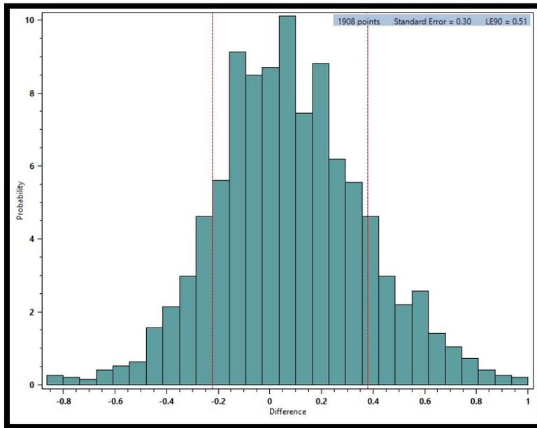
**Figure 11.** Histogram of the elevation differences between the Pleiades-1B stereo satellite elevations for the 14.4km by 13km area and all 1,908 elevation checkpoints. RMSE 30cm, LE90 51cm.
