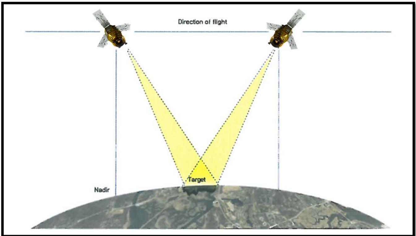
**Figure 2.** Illustration showing the process of taking satellite stereo photos. The satellite points forward to take the first photo. About one minute later, and 300km further along its orbital track, the satellite rotates to take the second photo looking backwards along the track. Hundreds of km<sup>2</sup> can be accurately surveyed with a single pair of stereo satellite photos.
