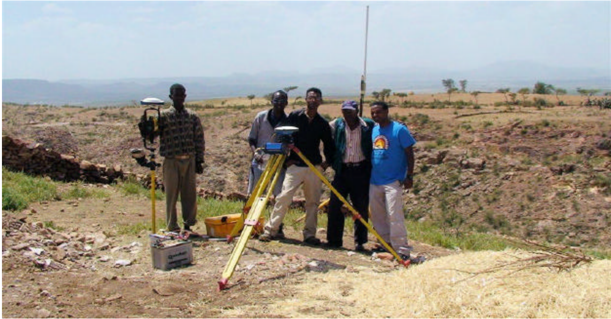
Figure 2. Asmara Project, Eritrea. MWH Geo-Surveys differential GPS survey crew and equipment. Over 45,000 gravity stations were surveyed from 2004 through 2008 using differential GPS instruments from Magellan. All of the GPS positions were surveyed in Real Time Kinematic (RTK) mode with accuracies of 2cm or better. 8,983 of these gravity survey stations were used as elevation checkpoints for the September 10, 2009 GeoEye-1 stereo satellite elevation mapping accuracy assessment. The Magellan RTK base with a ProMark TM 500 GPS rover are shown in this photo.
