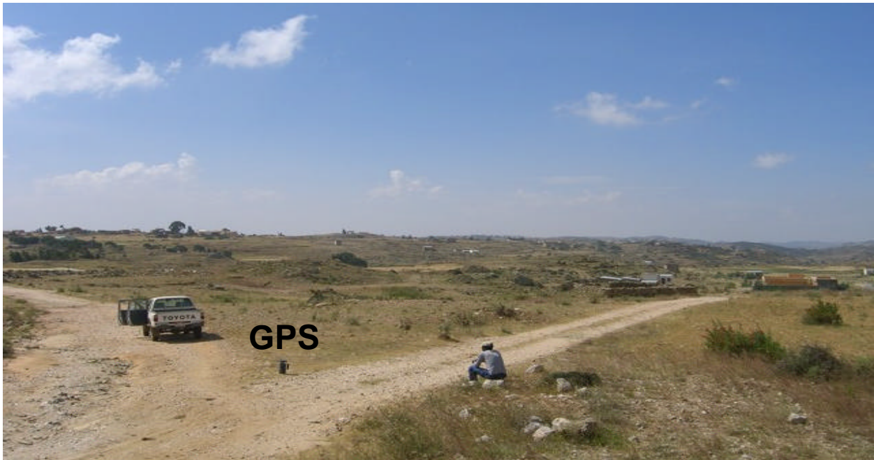
Figure 3. The entire 225 square kilometre Asmara, Eritrea, September 10, 2009, GeoEye-1 stereo satellite elevation mapping was referenced to the single ground control point shown in this photo. The 31cm RMSE accuracy of the stereo satellite elevation mapping was determined using 8,983 independent elevation checkpoints on slopes of less than 20% grade.
