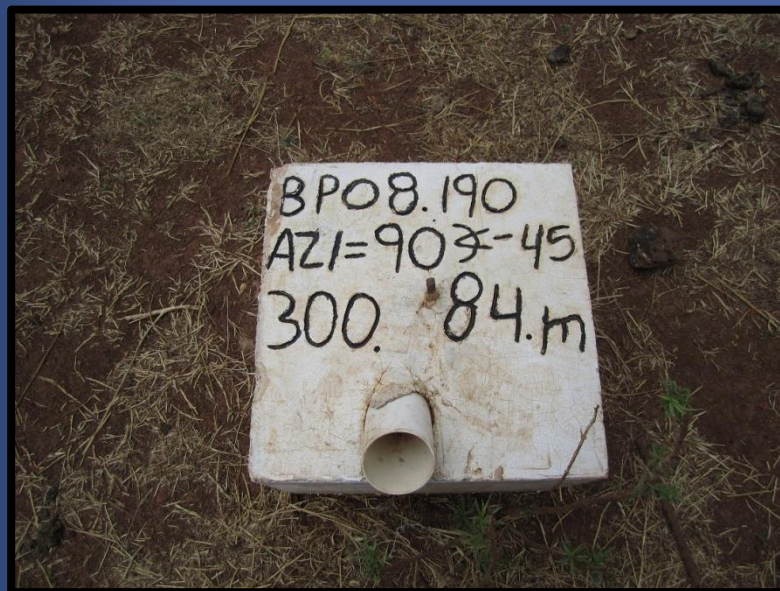
Drill hole collar 40cm x 40cm white concrete block
