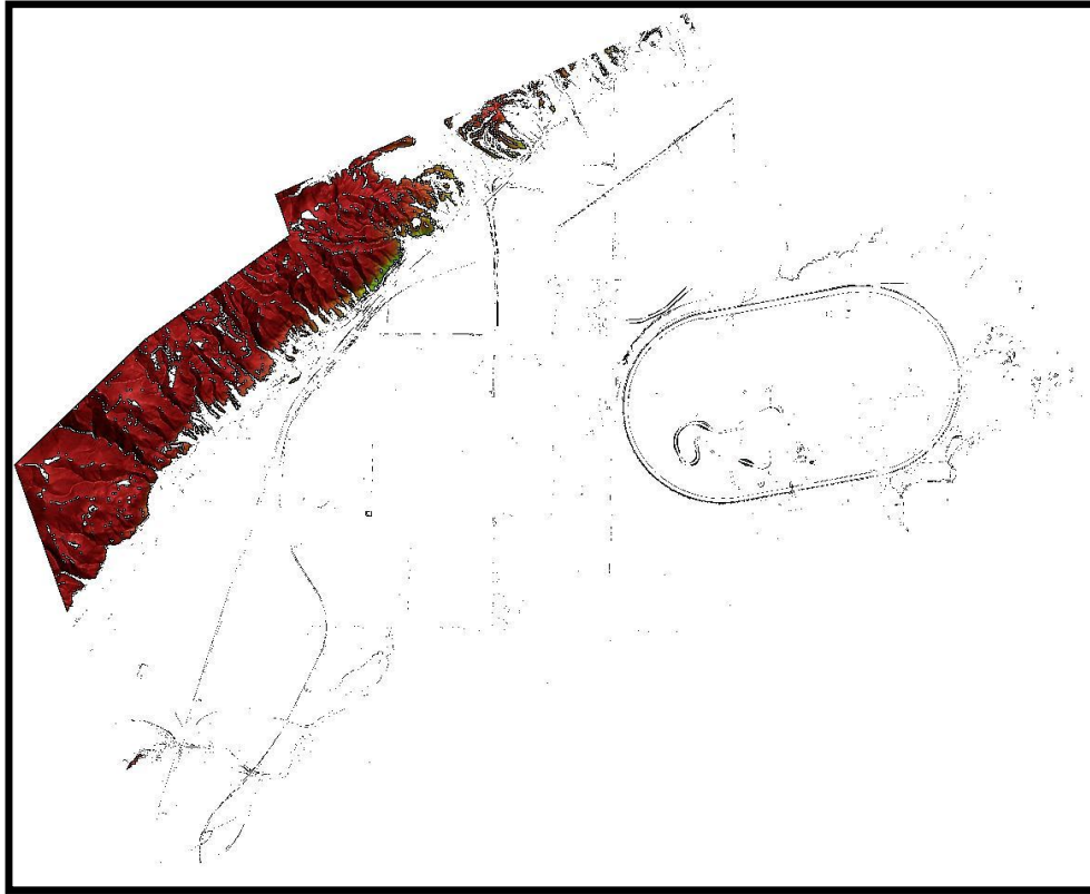
Figure 10. Stereo WorldView-2 DEM image covering the area of the LiDAR image in areas with slopes greater than 20% grade.
