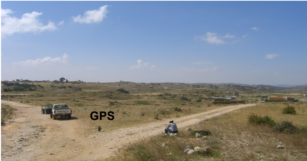
Figure 3. The entire 400 square kilometre Asmara, Eritrea WorldView-2 stereo satellite elevation mapping project was tied to two ground control points, one of which is shown in this photo. The accuracy of the stereo satellite elevation mapping of better than 30cm RMSE was determined using 21,944 independent elevation checkpoints.
