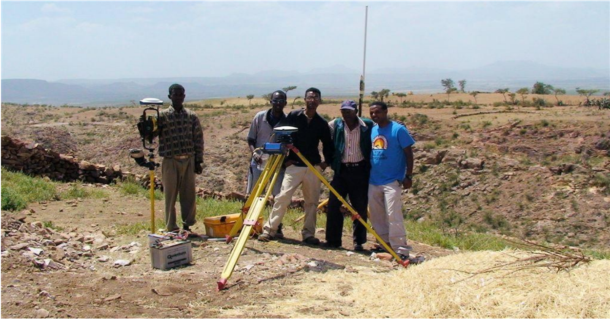
Figure 2. Asmara Project, Eritrea. MWH Geo-Surveys differential GPS survey crew and equipment. Over 45,000 gravity stations were surveyed from 2004 through 2008 using differential GPS instruments from Magellan. All of the GPS positions were surveyed in Real Time Kinematic (RTK) mode with accuracies of 2 cm or better. 21,944 of these gravity survey stations were used as elevation checkpoints for the WorldView-2 stereo satellite elevation mapping accuracy assessment. The Magellan RTK base with a ProMark™ 500 GPS rover are shown in this photo.
