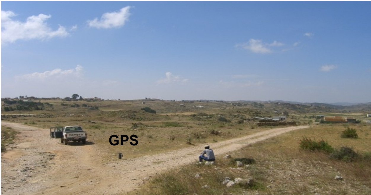
Figure 3. The entire 374 square kilometre Asmara, Eritrea WorldView-1 stereo satellite elevation mapping project was tied to the single ground control point shown in this photo. The accuracy of the stereo satellite elevation mapping of better than 35cm RMSE for areas up to 10km by 10km was determined using 15,020 independent elevation checkpoints.
