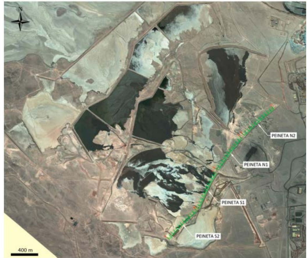
Figure 8 Plan of TSF showing N1 and N2, and S1 and S2 spigot distribution systems
